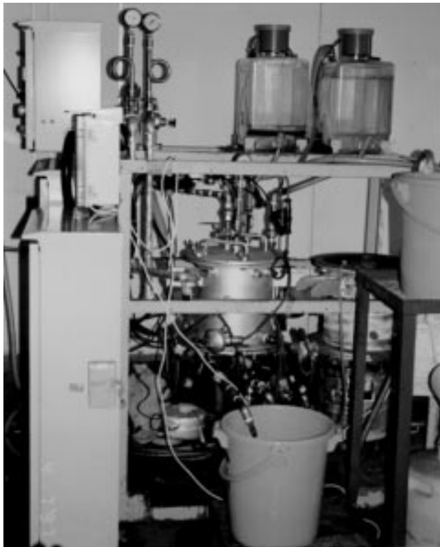
Fig. 1 Bench pilot corrosion test apparatus
