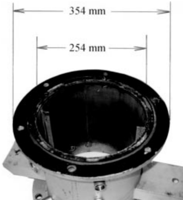
Fig. 7 Surface appearance of test vessel after immersion of 200 days
